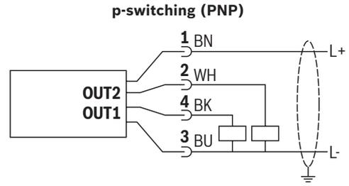
OUT1: Switching output or IO-Link
