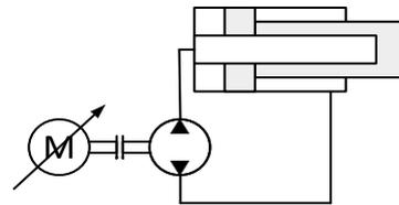
☞ The second pushing area is conventionally plugged and filled with nitrogen for preservation purpose. It can be utilized for applications where a static load is permanently present.
