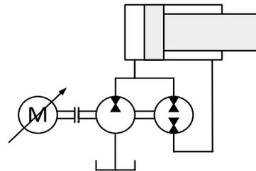
☞ In this situation, it has to be taken into account that the electrical grid is able to take the generated power from the electric motor, otherwise an brake resistor has to be used.
