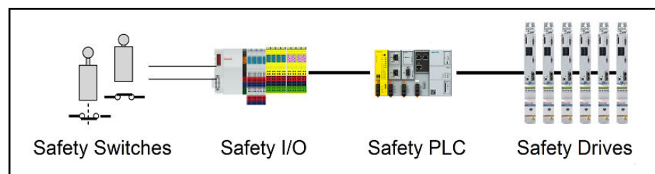
Fig. 4-12: Functional chain of logic operations from sensors to actuators
