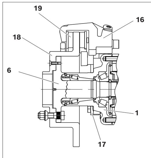
**Fig. 10: Dynamic disc (caliper) brake**
