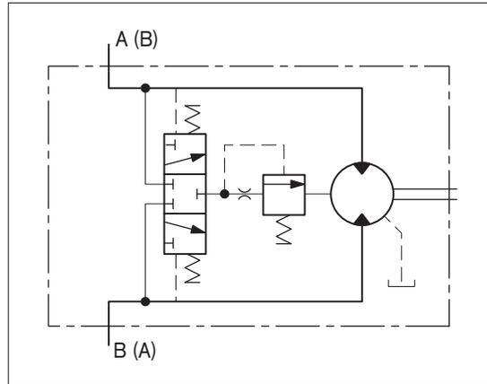
**Fig. 6: Flushing schematic**
