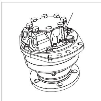
**Fig. 21: Speed sensor port (blanking plate fitted)**
