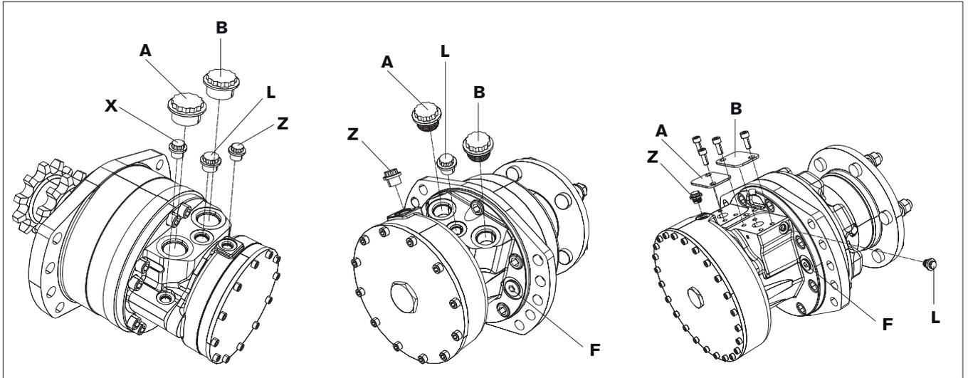
**Fig. 1: Radial piston motors with various port protection**
