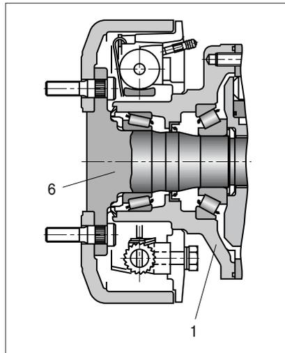
**Fig. 11: Dynamic drum brake section**
