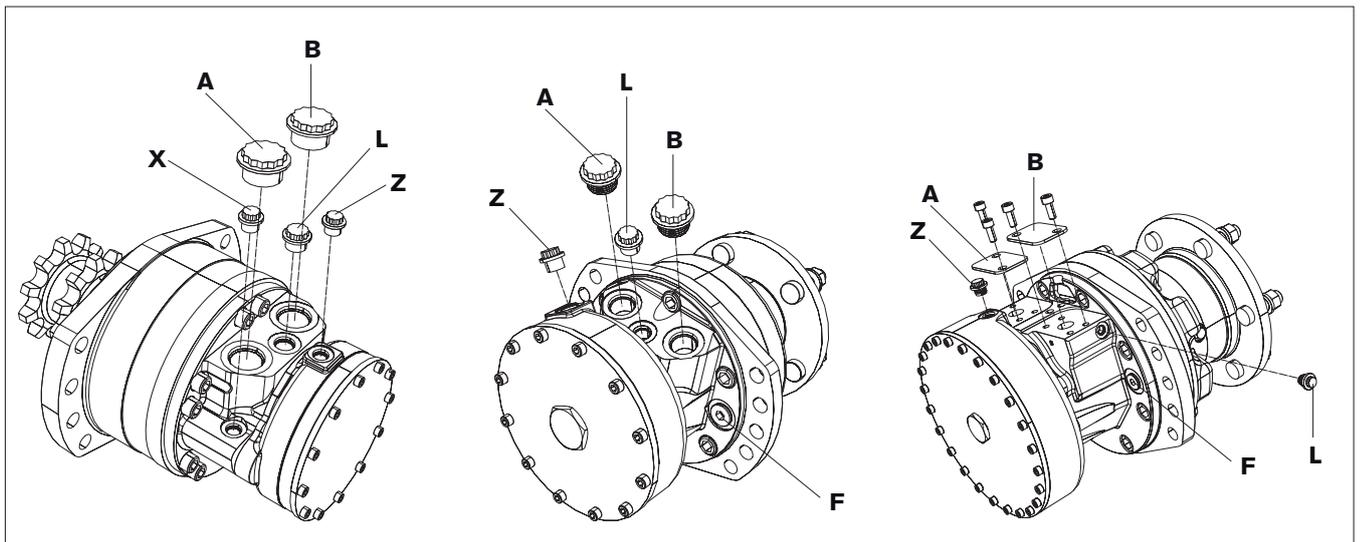
**Fig. 23: Removing transport protection**
