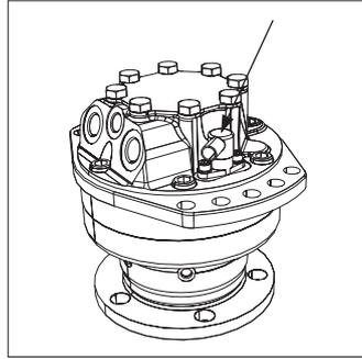
**Fig. 22: Tighten speed sensor to final torque**
