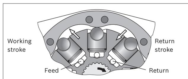
**Fig. 4: Torque generation**
