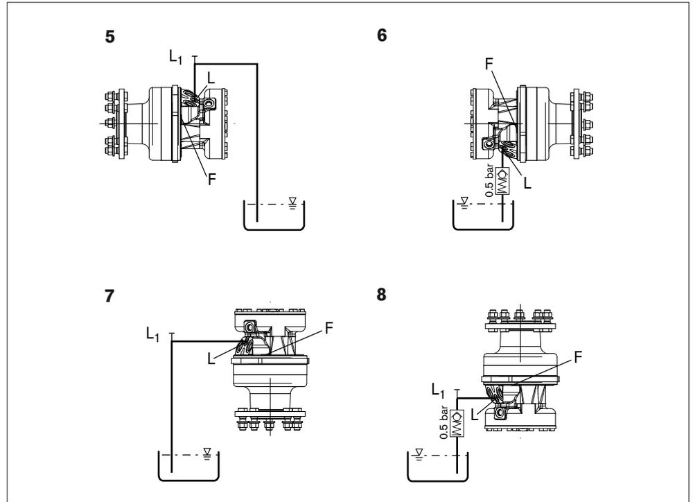
**Fig. 19: Above-reservoir installation MCR with installation position 7-12**
