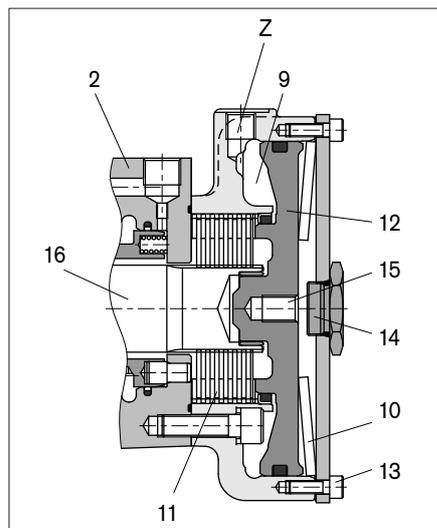
**Fig. 24: Holding brake section**
