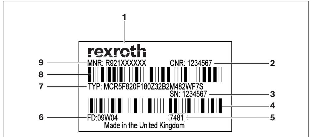
**Fig. 13: Label of a MCR motor**
