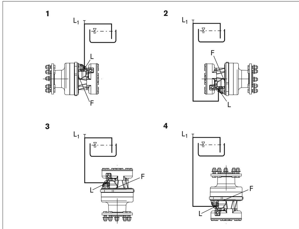
**Fig. 18: Below-reservoir installation MCR with installation position 1-4**
