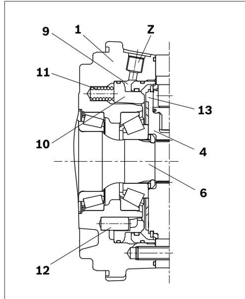
**Fig. 9: Holding brake section MCR-S**
