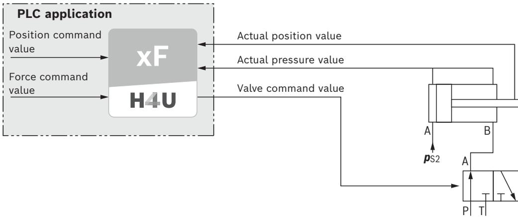
With the cylinder preloaded on the ring side, the load can be retracted and extended by pushing and pulling.
